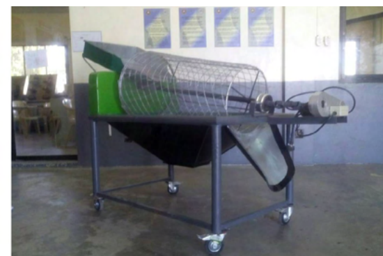
Figure 2. A Vibratory Rotary Sifter for Separating Granulated Materials
