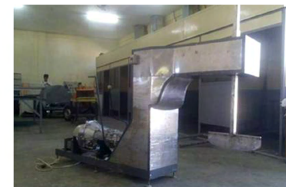
Figure 3. An Apparatus for Cooking Raw Sugarsuch as Muscovado and the Likes
